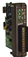
OL2258 High Speed Counter Single channel input. Pulse & Direction, Up/Down Count, or Quadrature. 0-80 KHz (0-160 KHz for Quad). Two high speed open collector outputs.
