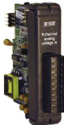
OL2408 Analog Voltage In 8-channel input, 0-5 or 0-10 VDC, 14-bit resolution.
