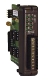
OL2109 DC Sinking 8-point, 0-40 VDC sinking output. 300mA sinking capability/point.
