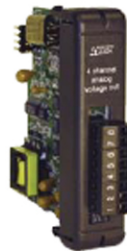
OL2304 Analog Voltage Out 4-channel output. 0-5V, 0-10V, +/-5V, +/-10V configurable. 12-bit resolution.
