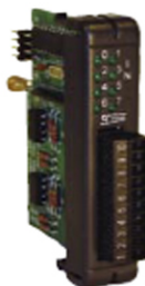
OL2208 DC Input 8-point, 10-30 VDC (sourcing or sinking).
