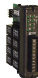
OL2108 Relay Output 8-point, 0-60 VDC or 0-120 VAC. 2A/point @ 24VDC, 1A/point @ 120VAC.
